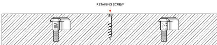
Use the **PEANUT® 2** without the 50mm screw for non-structural location and alignment of drawer fronts, side panels and other work pieces face to face.
